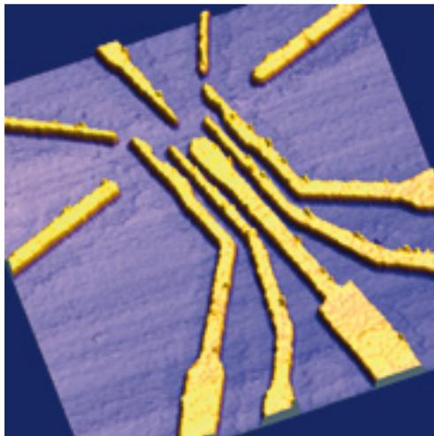
An atomic force microscope image of a double quantum dot nanostructure.
